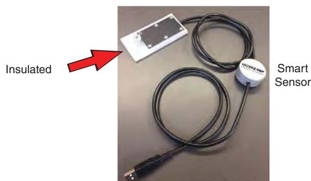
Figure 12.2b: UC202/IBP Temperature Smart Sensor with Insulated Black Panel (Black Standard)
