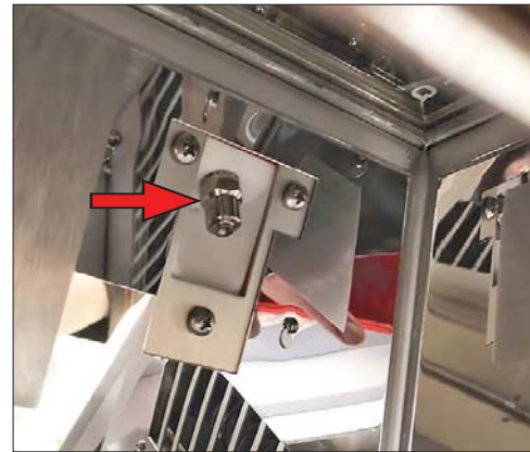
Figure 15.6.b: Interior of chamber showing right-side spray nozzle.
