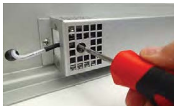
22. Make sure the trigger finger is in contact with the lamp but is not exerting excessive force .
