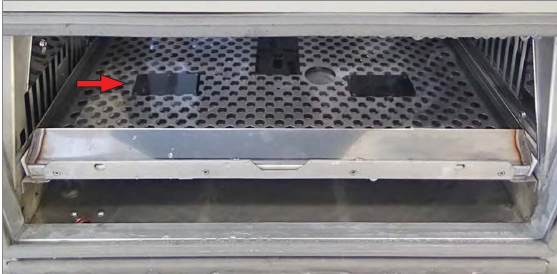
Figure 11.4s: Place specimens on the mesh insert.
