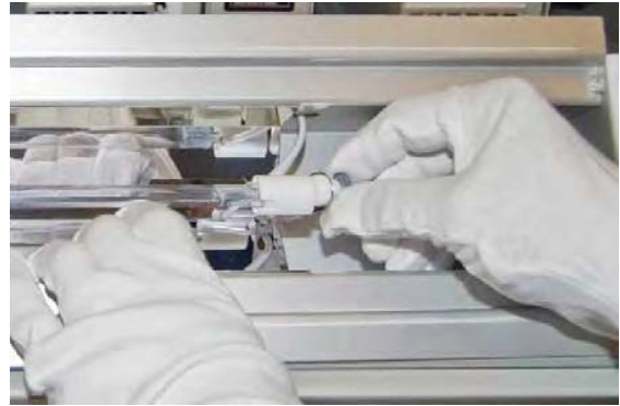
20. Install the new lamp in the housing. Guide the wires through the holes in the housing. Pull back the release lever to seat the lamp.
