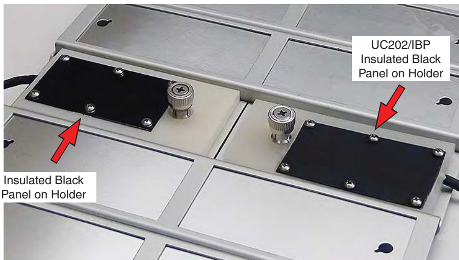
Figure 11.4k: Insulated black panel and UC202/IBP insulated black panel mounted on special holders.
