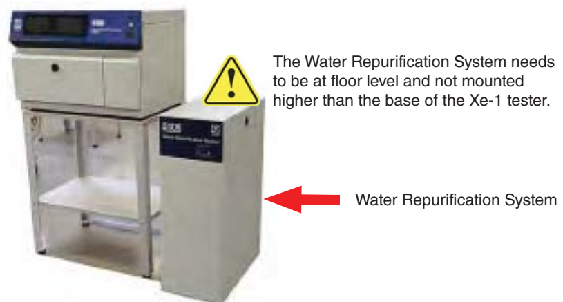
Figure 14.4: Q-SUN Xe-1 with water repurification system.
