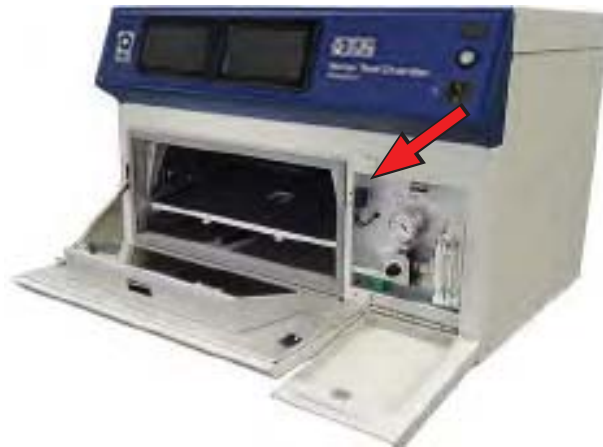
Figure 2.2: Xe-1 Chamber door interlock.
