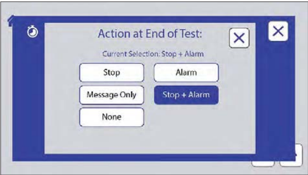
Figure 10.5c: Action at End of Test screen. Touch an action button to select that action.
