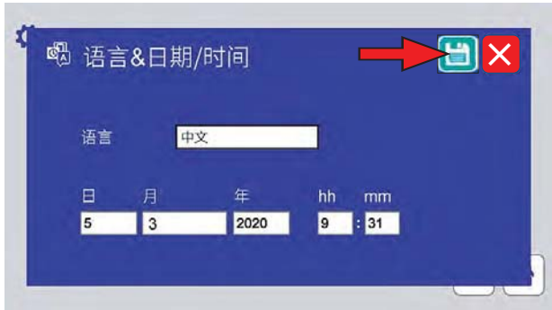
Figure 10.7l: All text on both screens will be in the selected language. Touch the save icon to save the selection.
