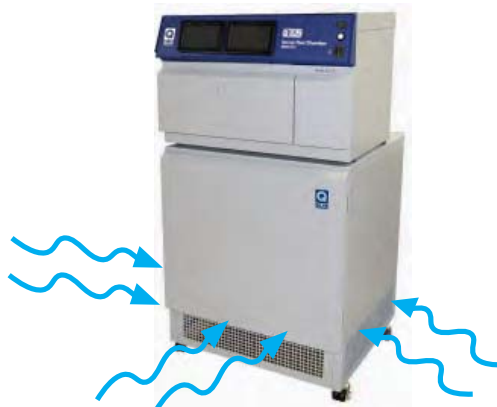
Figure 5.5.c: Q-SUN Xe-1-BCE and Xe-1-SCE chiller cooling air intake areas.
