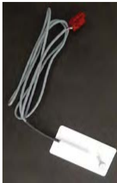
Figure 9.1d: Uninsulated white panel temperature sensor.
