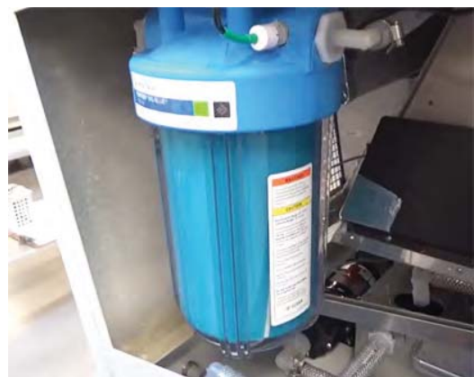
28. Check for water leaks around the housing cap. If any leaks, re-tighten the housing.
