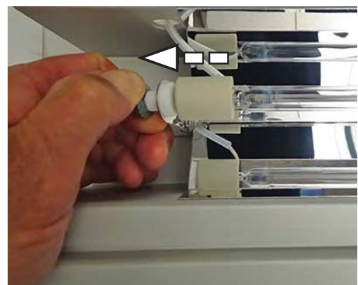
18. Release the lamp from the lamp housing by pulling lamp release lever away from the lamp.
