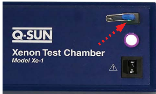
Figure 15.7.b: Connect the drive to the USB port on the Q-SUN control panel.
