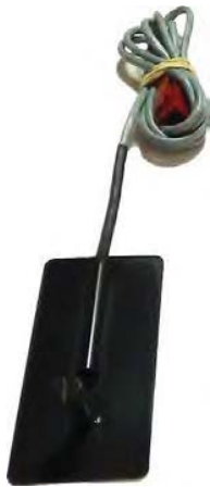
Figure 9.1a: Uninsulated black panel temperature sensor.
