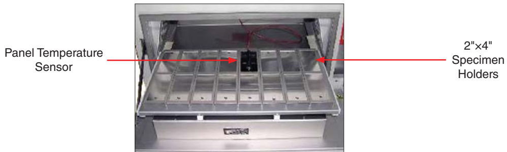
Figure 9.1f: Correct location of the Xe-1-SE, Xe-1-BCE and Xe-1-SCE panel temperature sensor.
