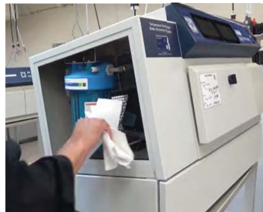
8. Place paper towels in the Xe-1-WE below the filter housing to absorb any spilled water.
