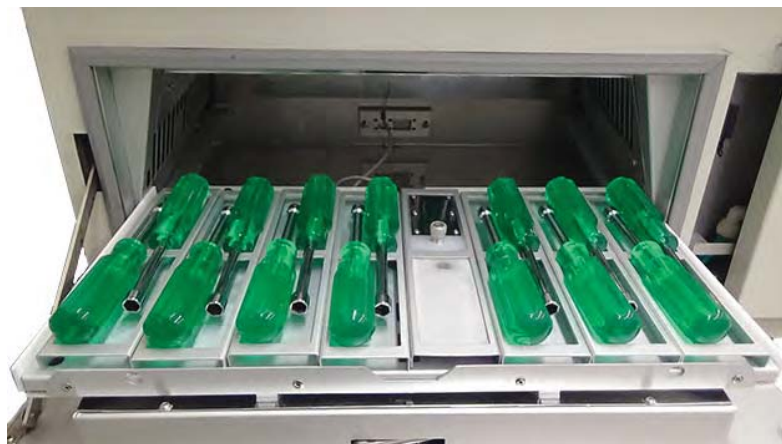
Figure 11.4e: Three dimensional specimens mounted in specimen holders.
