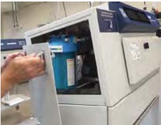
7. Remove the access panel. Set aside.
