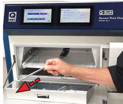
4. Lift the sensor out of the clip and carefully pull the sensor and cable out to the front of the machine.
