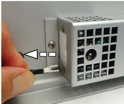
15. Pull the lamp wire through the hole to disconnect.
