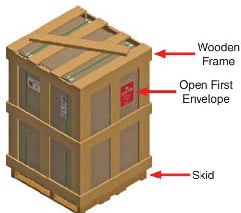
Figure 5.1.f: This packaging has a carton surrounded by a wooden frame fastened to a wooden skid.
