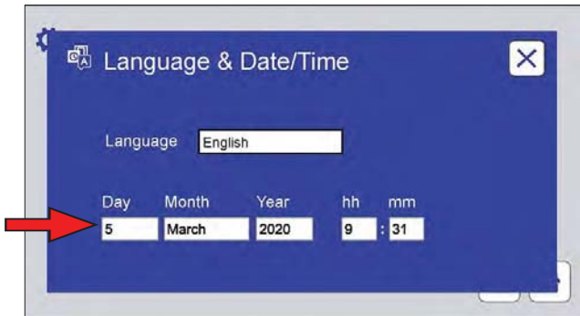
Figure 10.7m: This screen displays controls to set the date and time. Touch a text box to set Day, Month, Year, hh (hour) or mm (minute). hh display is always 24 hour time.
