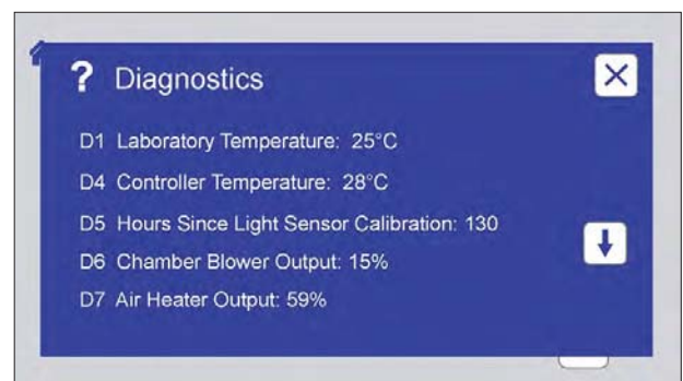
Figure 10.8b: The Diagnostics screen displays current machine operating conditions.
