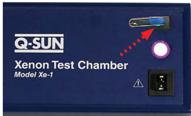
Figure 13.3b: Connect the drive to the USB port on the Q-SUN control panel.
