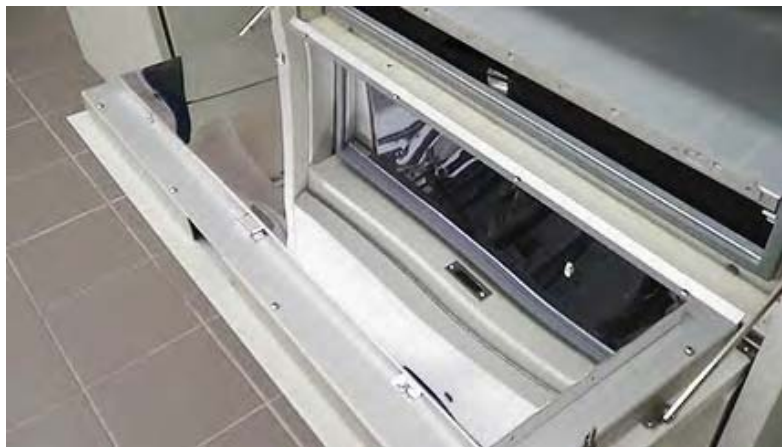
Figure 15.6.d: Clean Reflector - OK
