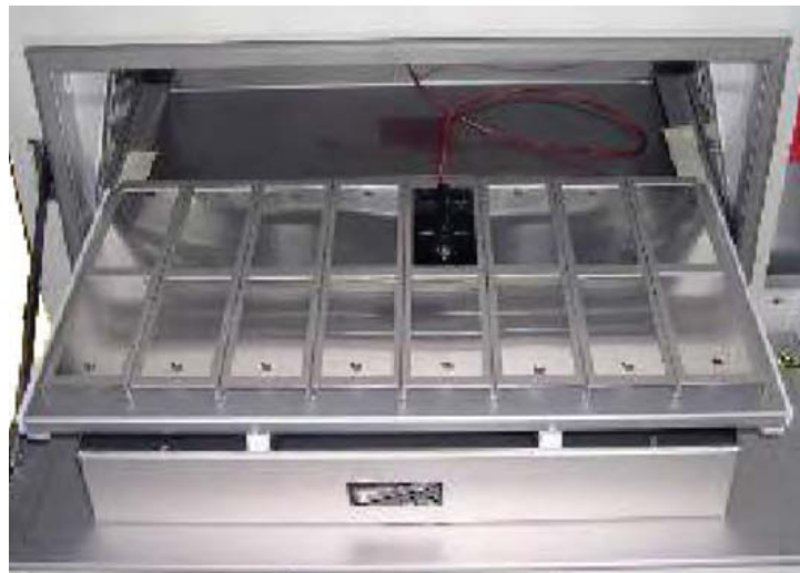
Figure 11.4g: Panel holder kit (X-10113-K) with eight (8) panel holders holding fifteen (15) 50×100 mm (2"×4") specimens and one (1) black panel.
