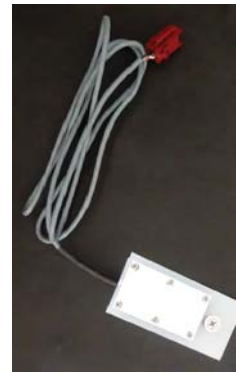
Figure 9.1e: Insulated white panel temperature sensor.
