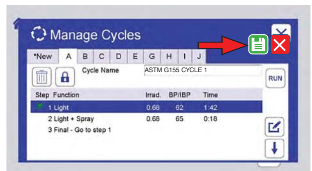
Figure 10.6.5f: The edited step is shown for the cycle. Touch the save icon to save the edited cycle. NOTE: pre-programmed test cycles cannot be edited.
