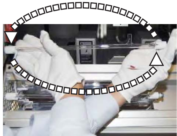
Figure 16.3.b: Swap ends to reverse the lamp and reinstall.
