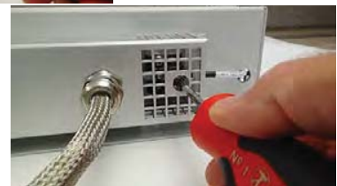
23. Reconnect the lamp wires. Tighten the screws.
