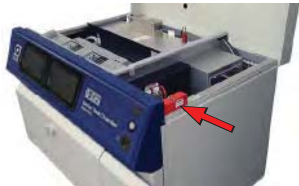
Figure 2.1d: Interlock switch location (lid open).
