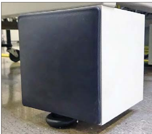
Figure 14.2.b: Riser installed with leveling foot.
