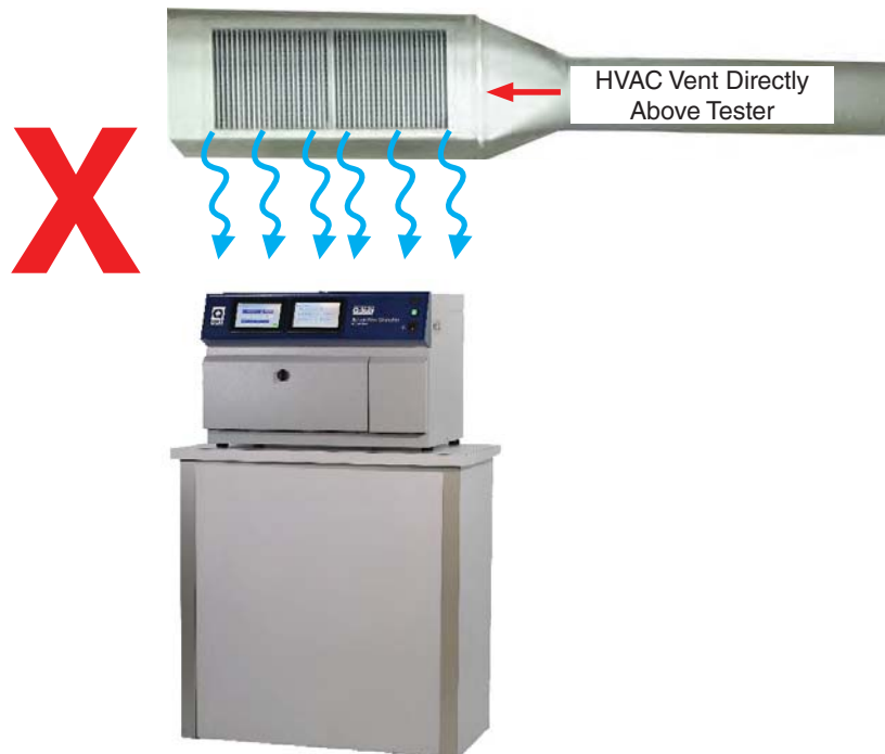
Figure 4.2d: Keep tester away from sources of hot or cold air.
