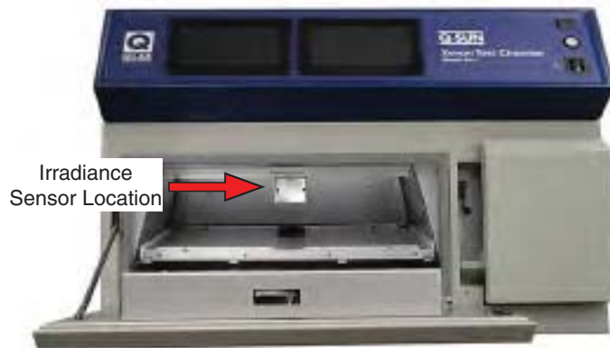
Figure 6.3a: Xe-1 Irradiance sensor located on rear chamber wall (behind shield).
