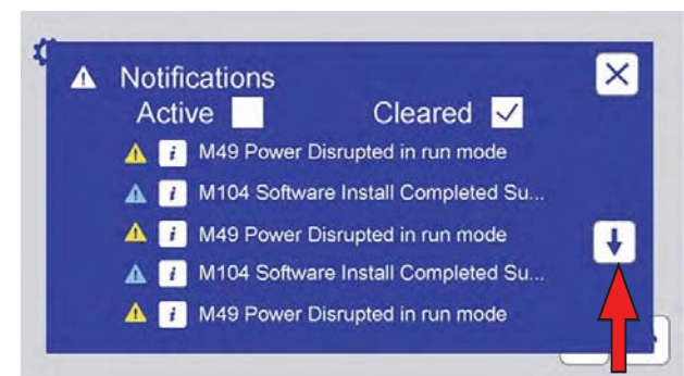
Figure 10.4d: Touch the scroll button(s) to move down or up the notification list.
