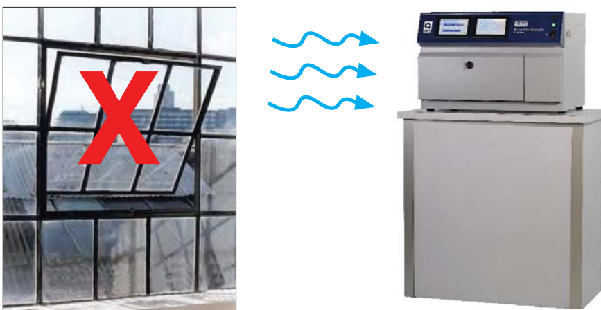
Figure 4.2c: Do not locate testers near open windows.
