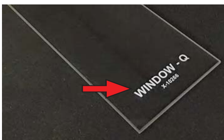
Figure 11.3e: Optical filter type etched into filter.
