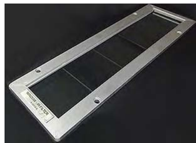
Figure 11.3f: Multi-segment optical filter in frame.
