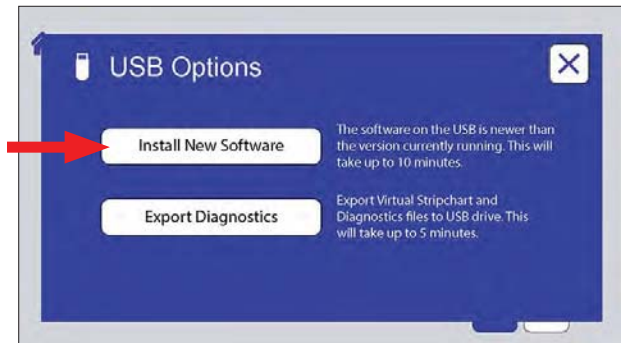
Figure 15.7.c: The USB Options screen displays the software installation button.
