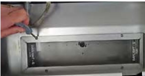
Figure 11.3c: Unscrew UV filter frame.
