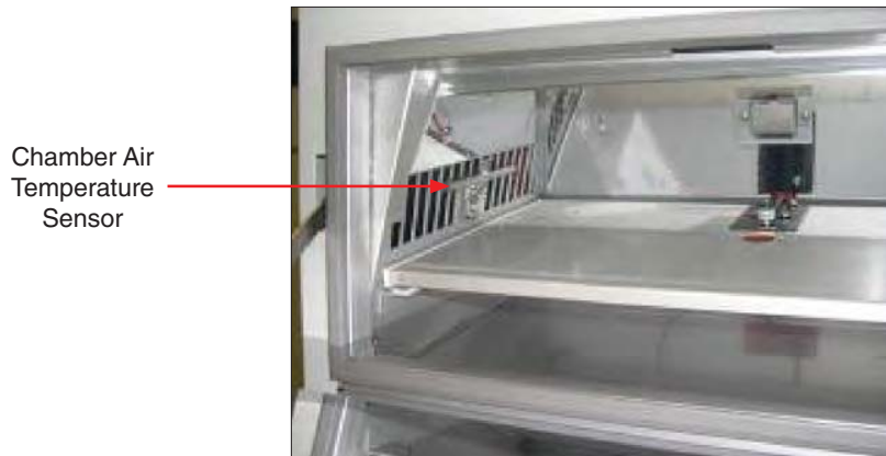
Figure 9.2: Chamber air temperature sensor location in Xe-1-BCE and Xe-1-SCE test chambers.
