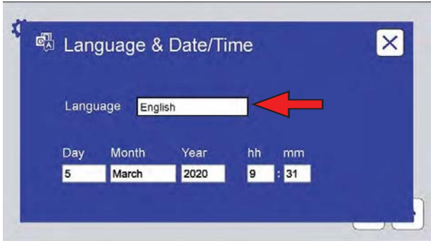
Figure 10.7i: This screen displays controls to select the control interface language.
