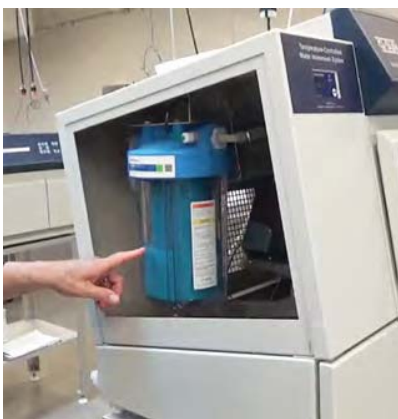
27. Allow the filter housing to fill with water.
