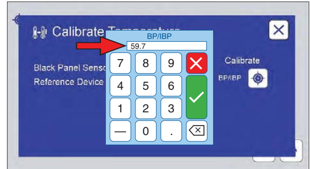
6. Use the keypad to enter the reference temperature into the reference device text box.
