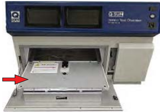
Figure 11.4a: Specimen tray without clips (X-10195-X).
