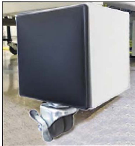
Figure 14.2.c: Riser installed with caster.
