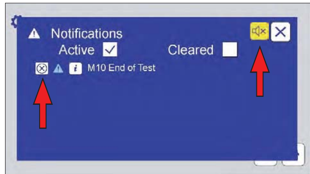
Figure 10.4h: If the alarm is active, touch the yellow mute icon to silence. When the notification has been resolved, touch the icon to the left of the notification to clear it.
