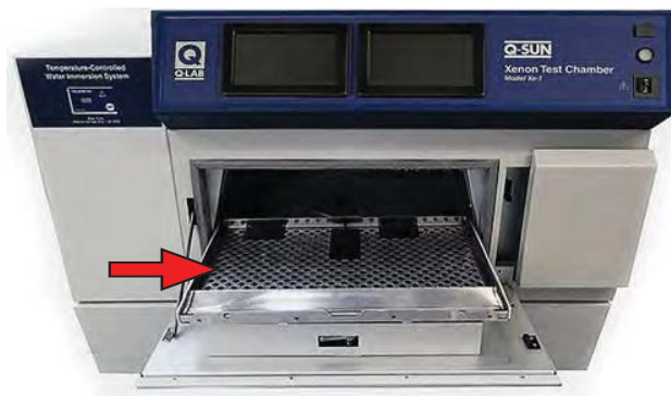
Figure 11.4b: Xe-1-WE with ponding tray mounted on specimen tray.
