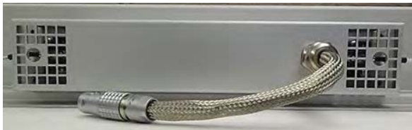
13. Locate the center hole in each end of the lamp housing cover.
