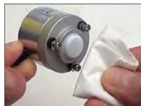
Figure 12.1e: Clean the sensor face with alcohol and a soft cloth.
