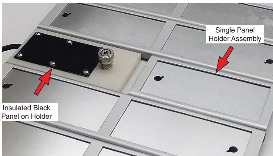
Figure 11.4j: Insulated black panel mounted on special holder and single panel holder with (1) 50×100 mm (2"×4") specimen.
