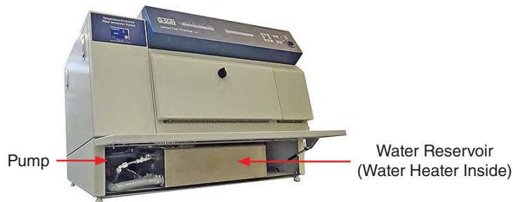
Figure 8c: Lower door open showing reservoir and pump.
