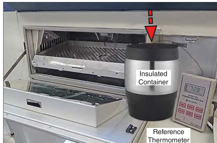
Figure 12.2f: Place the Xe-1-WE panel temperature sensor and the reference thermometer in an insulated container of water.
