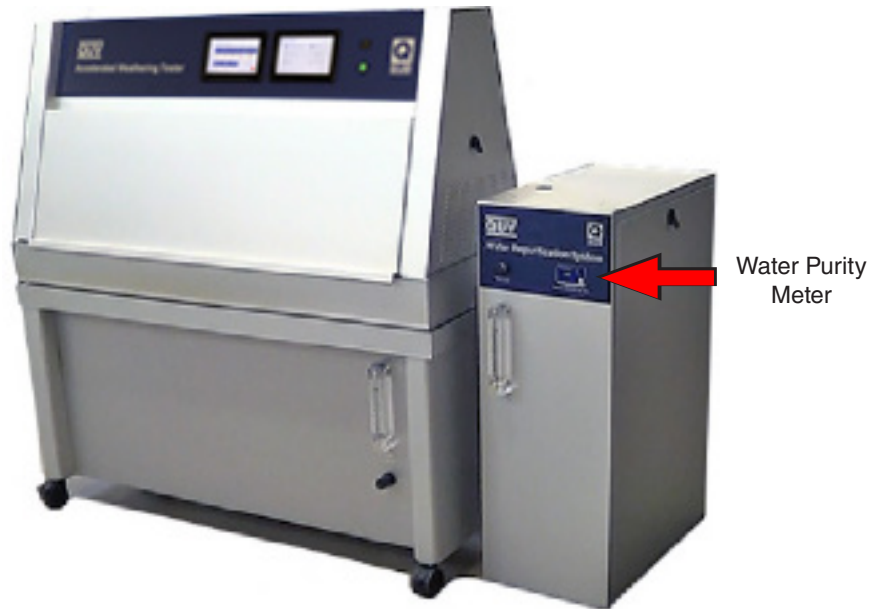
Figure 13.3c: QUV with standalone water repurification system (part no. V-60160-K)
