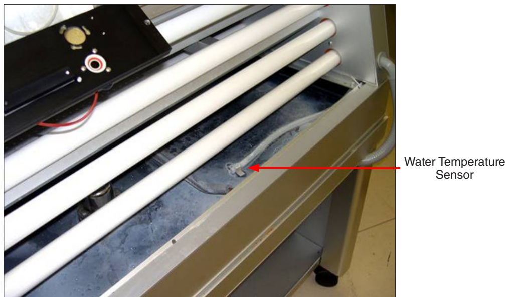
Figure 8.3: Water temperature sensor location (shown with water pan cover removed).
