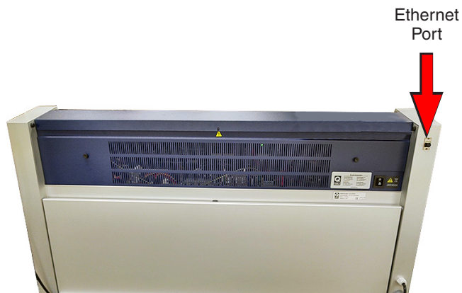
Figure 12.1: Ethernet port located on right rear of tester frame.
