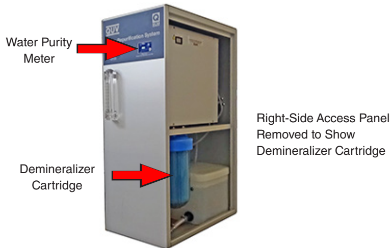
Figure 14.5c: Stand-alone water repurification system.
