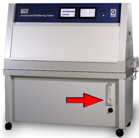
Figure 13.3b: Flow adjustment valve and flow meter location.
