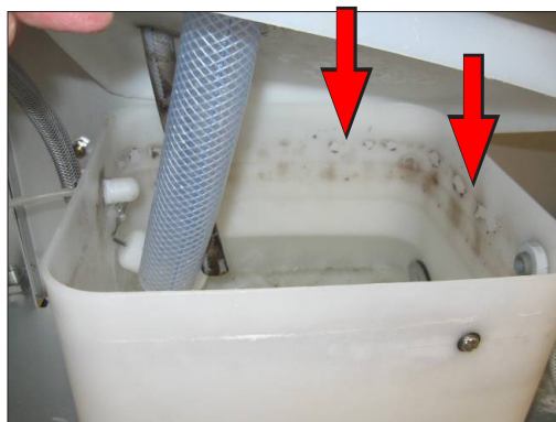
Figure 14.5g: Reservoir lid removed showing mold growth.
