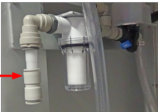
Figure 5.4f: Tube adapter for 12 mm water supply tube.
