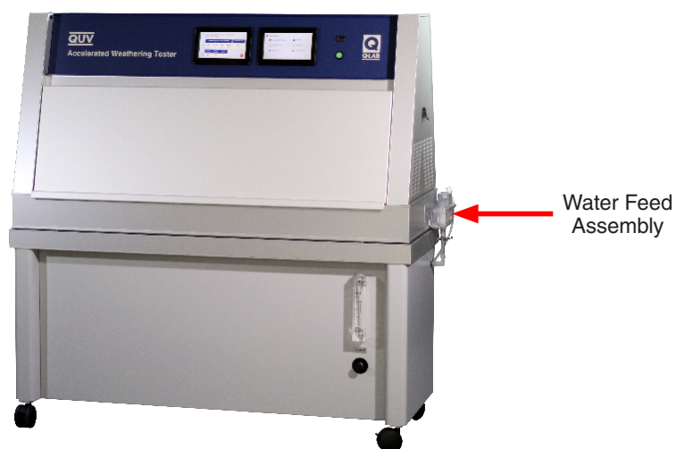
Figure 5.4a: QUV water supply connection location.
