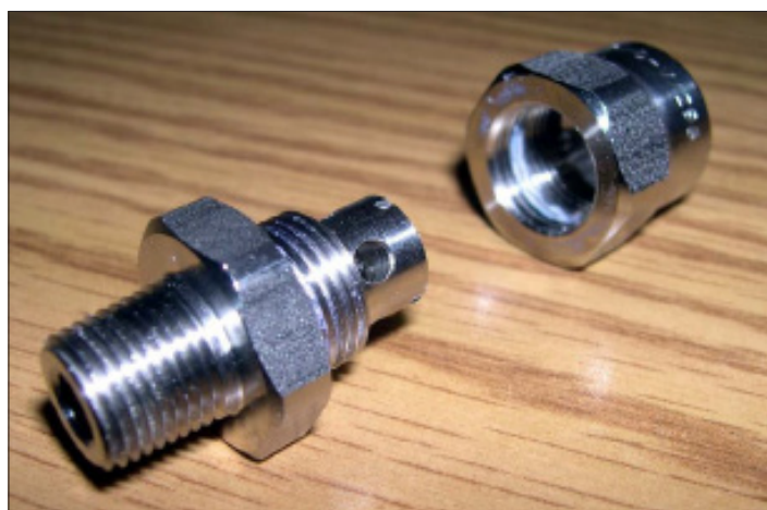
Figure 14.3b: Spray nozzle disassembled for cleaning.
