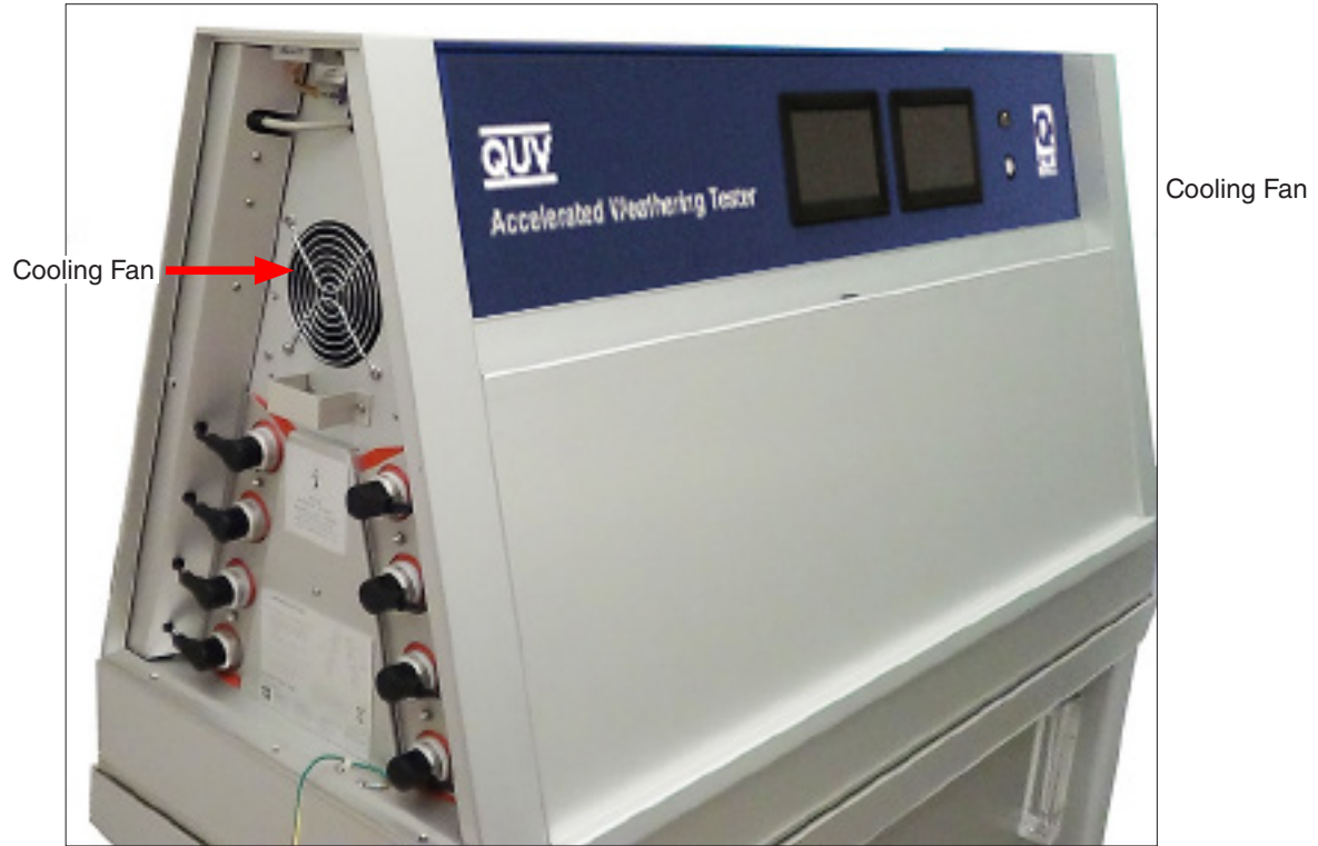
Figure 6.3: QUV left end cover removed showing cooling fan.
