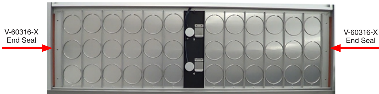
Figure 10.3a: QUV front view with 75 mm (3") wide specimen holders.
