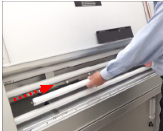
12. Hold the lamp and carefully slide it to one end until it pulls out of the lamp gasket.
