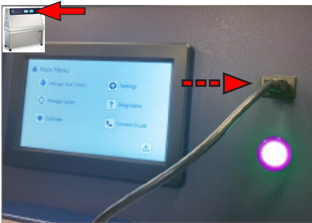
3. Plug the Smart Sensor into USB connector on the QUV control panel.
