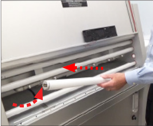
13. Carefully rotate the lamp outward, slide out of the other lamp gasket. Remove the lamp.
