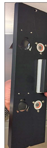
Figure 8.1d: Interior of black panel showing insulated temperature sensor.
