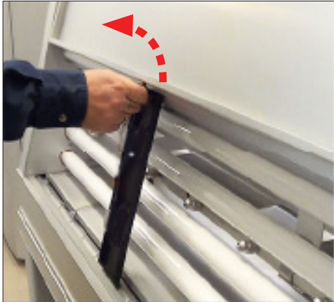
7. Loosen the thumb screws at the top of the detector panels on the QUV tester.
