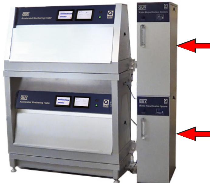
Figure 13.3d: Water repurification systems (V-60160-K × 2) stacked for QUV/spray testers on space saver frame.
