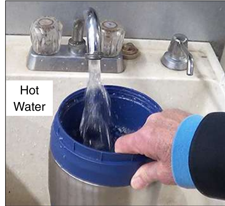
16. Fill the container to 20 mm below the top with hot water. The water should be approximately the same temperature as the highest temperature programmed in the test cycle.
