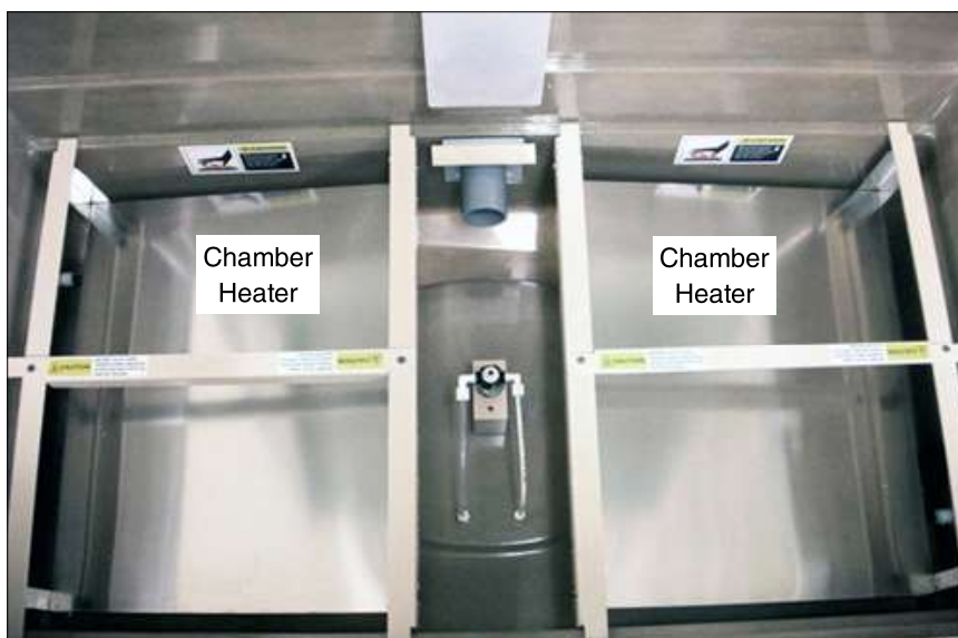
Figure 8.6: Chamber heater location at bottom of chamber (diffuser plates removed).
