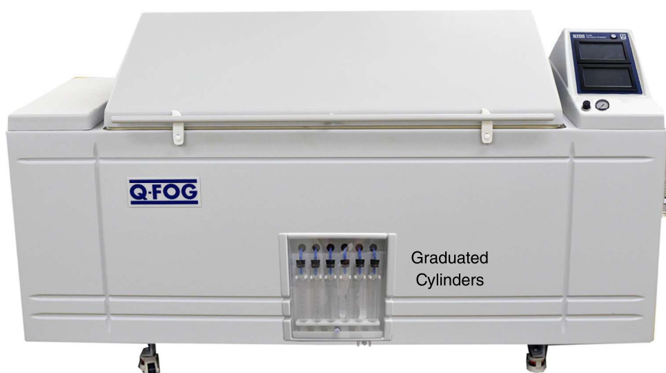
Figure 12.2d: External collection cylinders on chamber front.
