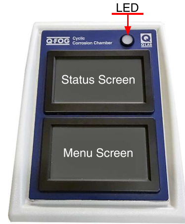
Figure 9.1b: Touch-screens and LED location on control top.
