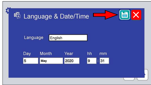
Figure 9.7p: Touch the save icon to save any changes to the Language & Date/Time. NOTE: The controller does not automatically adjust for Daylight Savings Time.
