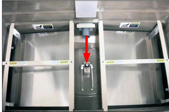
Figure 8.8a: Fog spray nozzle located at bottom of test chamber (diffusers removed).
