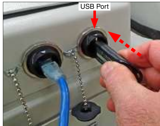
Figure 13.3b: Connect the drive to the USB port at the rear of the Q-FOG control top.
