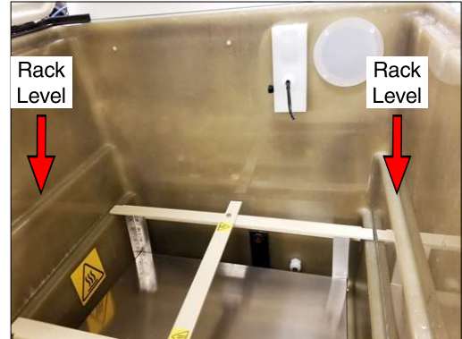
Figure 10.2f: Chamber interior showing rack grate mounting level
