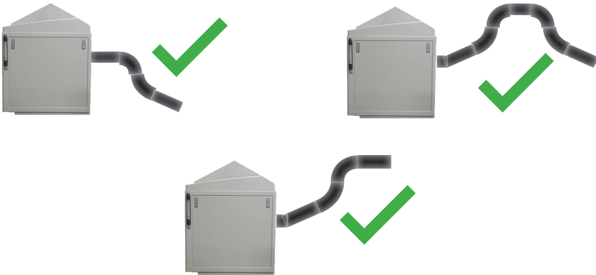
Figure 6.7f: Correct vent installations.
