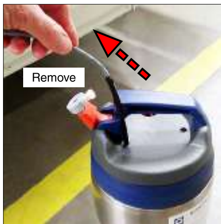
45. Remove the chamber temperature sensor from the insulated calibration container. Dry the sensor
