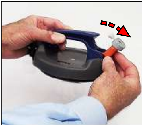
17. Rotate the reference thermometer fitting away from the handle on the insulated calibration container lid.
