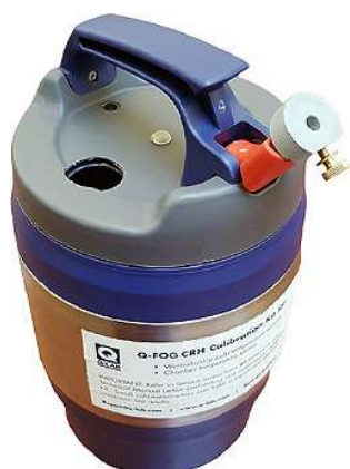
47. Empty the water from the insulated calibration container and replace the lid. Save the insulated calibration container for future calibrations.
