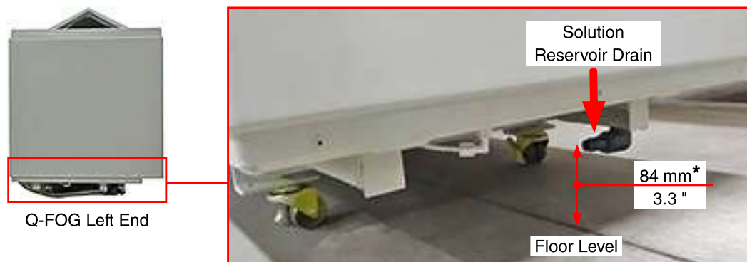
Figure 6.6d: Solution reservoir drain location with 70 mm (2.75") high optional caster.
