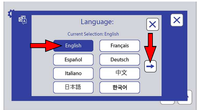
Figure 9.7j: Touch the language text box to select the control display language. Touch the Down Arrow icon to display additional available languages.
