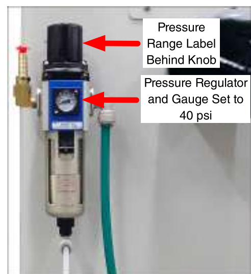
Figure 6.4b: Compressed air pressure regulator.
