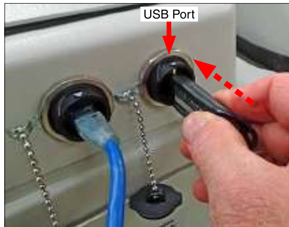
Figure 14.4c: Connect the drive to the USB port at the rear of the Q-FOG control top.
