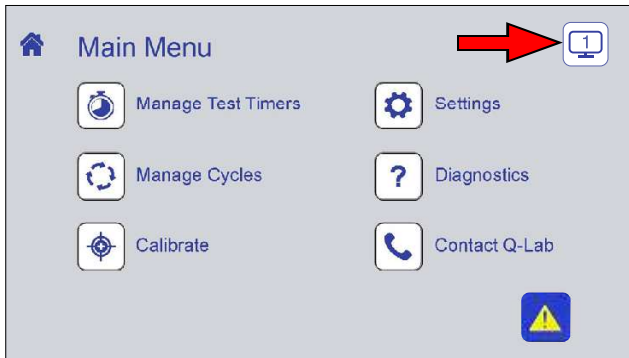
Figure 9.7x: Main Menu in single screen mode. Touch the screen icon.
