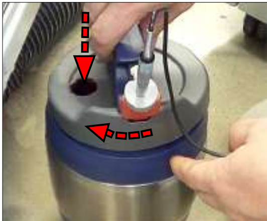
21. Replace the lid on the insulated calibration container. Tighten the lid.
