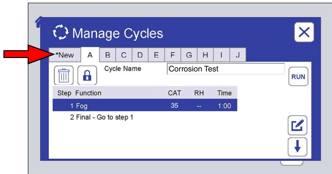
Figure 9.6.7a: To create a new cycle, touch the *New tab.
