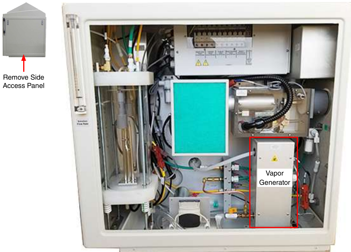
Figure 8.3: Access panel removed to show vapor generator.
