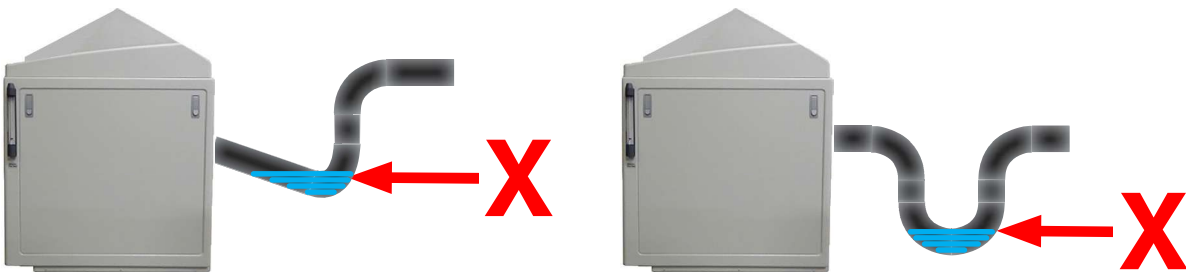
Figure 6.7g: Incorrect vent installations.
