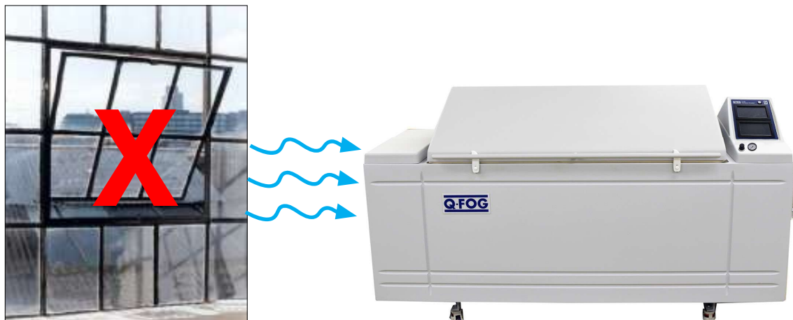
Figure 4.2c: Do not locate Q-FOG near open windows.
