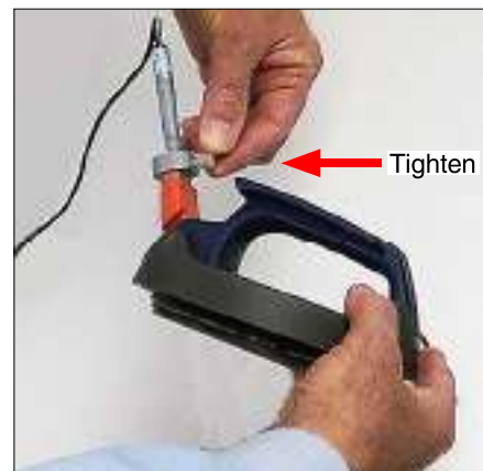
20. Hand tighten the reference thermometer fitting thumbscrew to hold the reference thermometer sensor in place.
