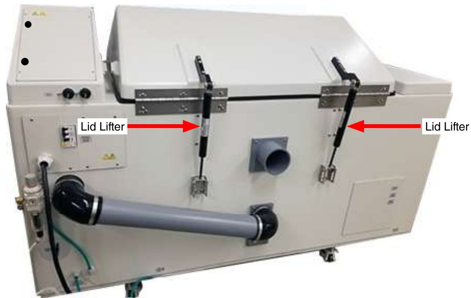
Figure 8.12a: Q-FOG rear view showing lid lifters.
