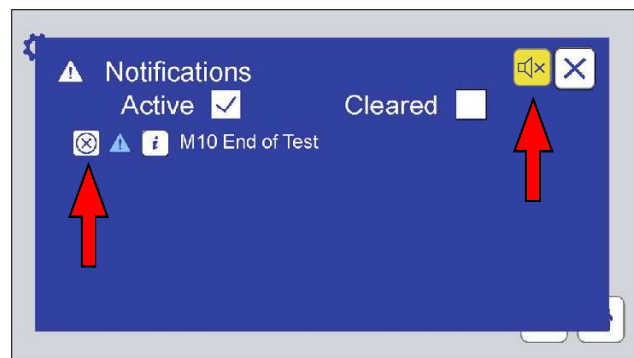
Figure 9.4h: If the alarm is active, touch the yellow mute icon to silence. When the notification has been resolved, touch the icon to the left of the notification to clear it.
