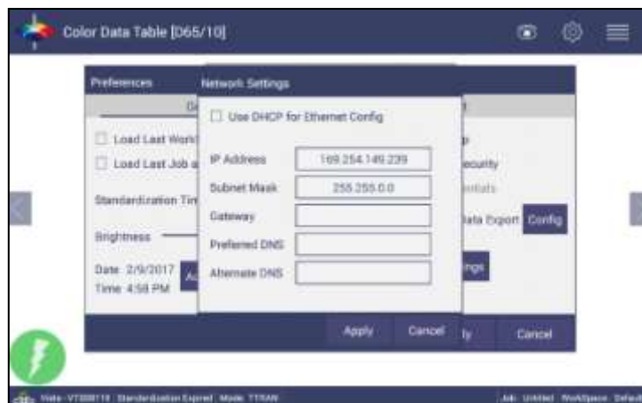
Figure 105. Configure IP Address & Subnet in Essentials
