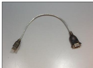
Figure 90- RS-232 to USB converter for connection via USB port
