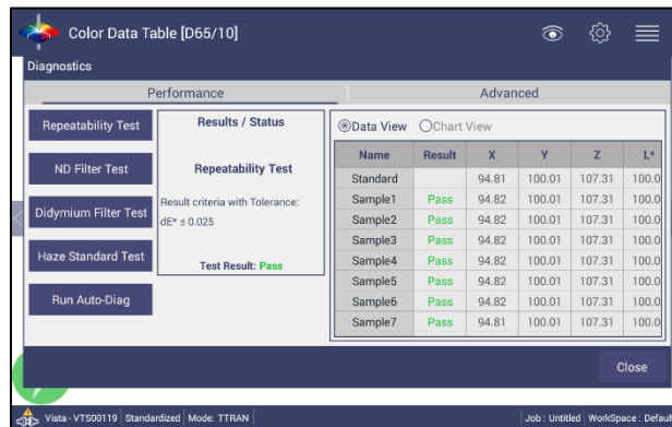
Figure 64. Read Options to select Pass/Fail and Tolerances
