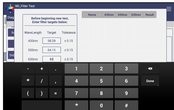
Figure 65. Input Target Values for ND Filter
