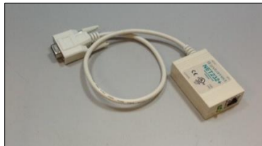
Figure 89- Ethernet to RS-232 converter for Connection via Serial port
