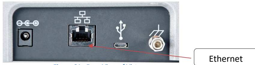
Figure 91. Rear View of Vista
